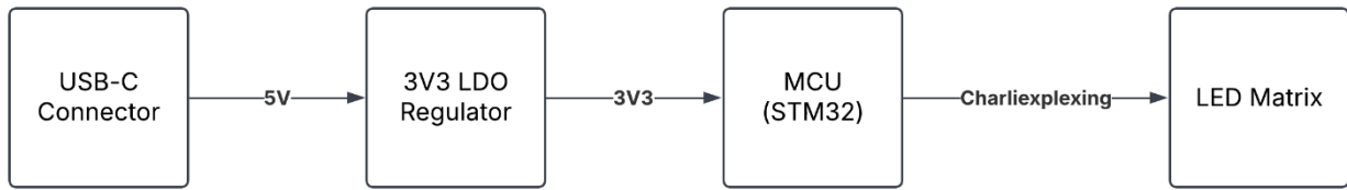
Figure 1: Blocks diagram of the initial design
